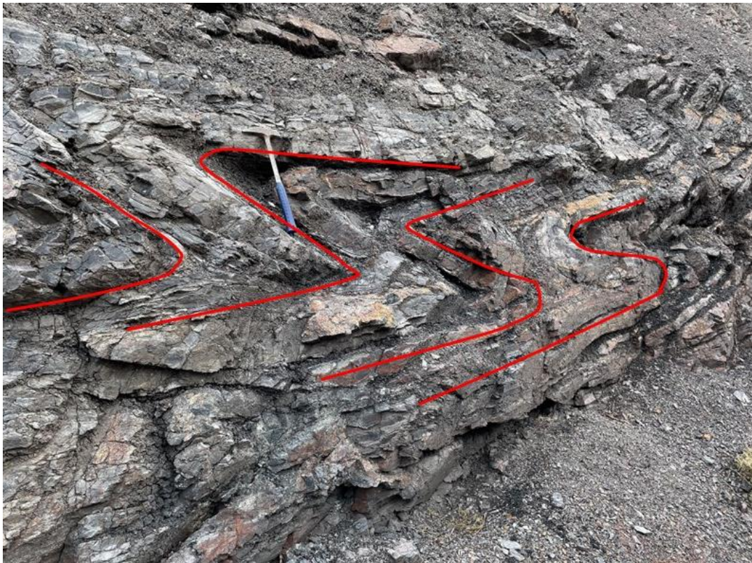
Figure 9. North-viewing photo of folded upper plate cherty mudstone exposed in a trench cut at the Iron Point vanadium deposit. Fold axes trend 040°-045° and plunge 11°-15° to the northeast. Hydrothermal alteration includes, carbon, clay, quartz veins and hematite. Photo taken at UTM coordinate N45303070 E473279.
