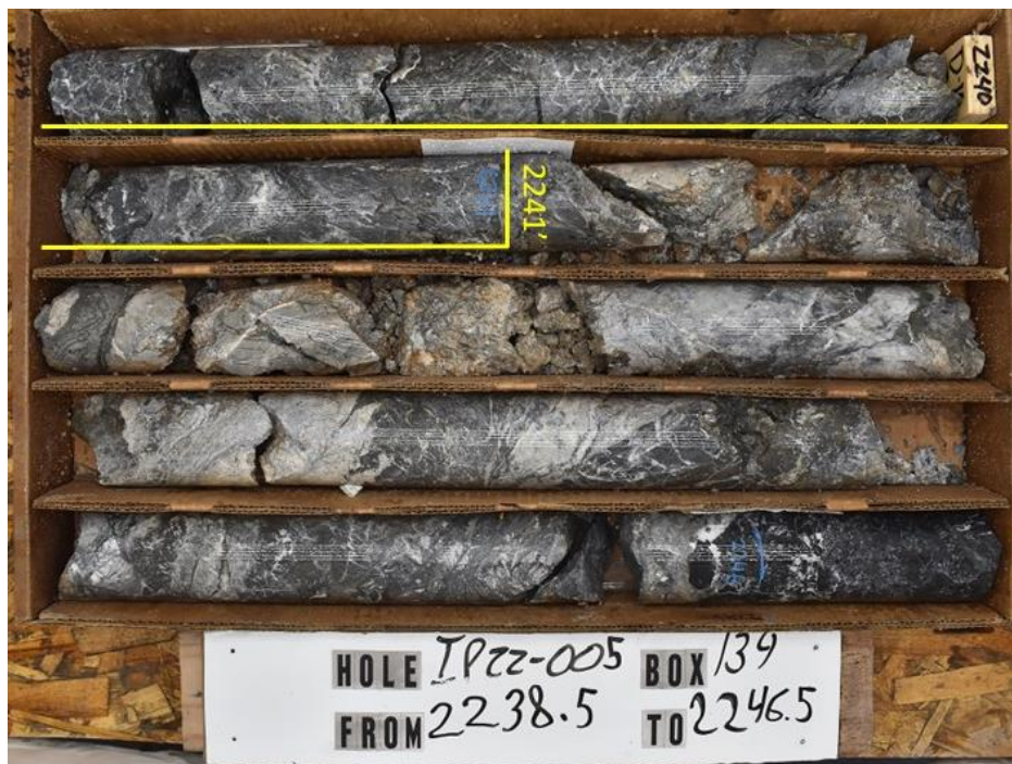
Figure 40. HQ core from drill hole IP22-005. The interval from 2236 to 2241 feet (681.5 to 683.1m) assayed 3.11 g Au/t in decalcified, weakly silicified, pyritic multilithic breccia.
