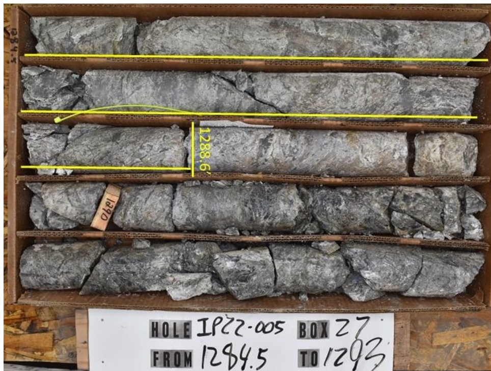
Figure 39. HQ core from drill hole IP22-005. The interval from 1283 to 1288.6 feet (391.1 to 392.8m) assayed 12.30 g Au/t in bleached, sheared/brecciated and clay altered intrusive with limestone clasts.
